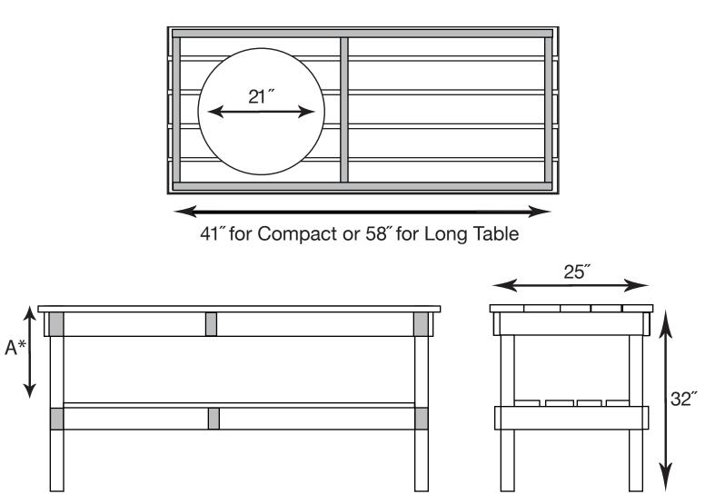
A\* is the measurement from the top of the lower shelf to the top of the table. The "A" measurement is 15"
